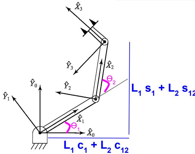
$$x = L_1 c_1 + L_2 c_{12} = L_1 c_1 + L_2 c_1 c_2 - L_2 s_1 s_2 = (L_1 + L_2 c_2) c_1 - (L_2 s_2) s_1$$
