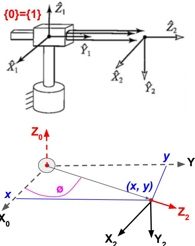
Given  ${}^0_2\mathbf{T} = \begin{bmatrix} {}^0_2R & {}^0P_{2org} \\ \hline 0 & 1 \end{bmatrix} = \begin{bmatrix} \sin \phi & 0 & \cos \phi & x \\ -\cos \phi & 0 & \sin \phi & y \\ 0 & -1 & 0 & 0 \\ 0 & 0 & 0 & 1 \end{bmatrix}$
