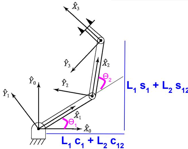
$$\begin{aligned} {}^0_3\mathbf{T} &= {}^0_1\mathbf{T} \cdot {}^1_2\mathbf{T} \cdot {}^2_3\mathbf{T} \\ &= \begin{bmatrix} c_{123} & -s_{123} & 0 & L_1 c_1 + L_2 c_{12} \\ s_{123} & c_{123} & 0 & L_1 s_1 + L_2 s_{12} \\ 0 & 0 & 1 & 0 \\ 0 & 0 & 0 & 1 \end{bmatrix} \equiv \begin{bmatrix} c\phi & -s\phi & 0 & x \\ s\phi & c\phi & 0 & y \\ 0 & 0 & 1 & 0 \\ 0 & 0 & 0 & 1 \end{bmatrix} \end{aligned}$$
