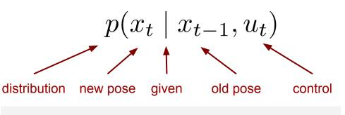
Robot motion 'rules' given current state & control input
