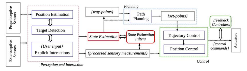
**<u>Pipeline Example:</u>** autonomous target following by mobile robots
