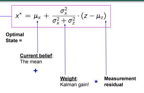
The **Kalman gain** determines how much your estimate needs to change given a measurement
